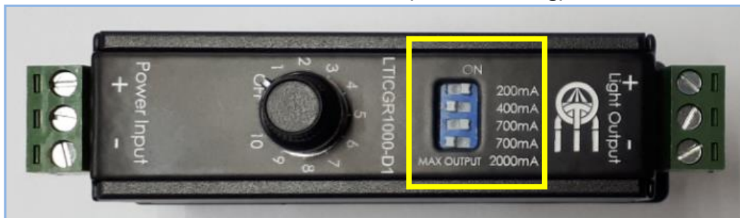
DIP SWITCH (Current Setting)
