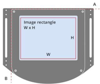
The width of the FOV (W) is aligned along the A axis. The height of the FOV (H) is aligned along the B axis.
