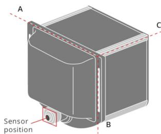
The long side of the sensor has to be aligned along the A axis.
