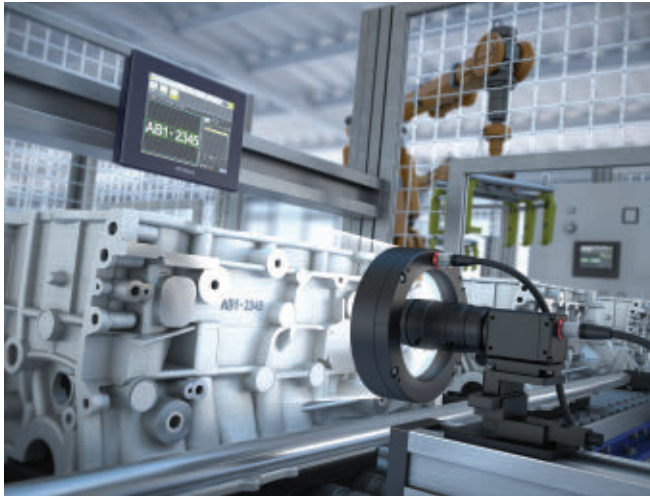
Figure 2: LumiTrax technology is designed to enable stable inspection—rejecting bad parts without sacrificing production output—where changes in the target’s surface exist, but with very little visible contrast.
