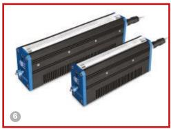
inspection system that enables fast, reliable defect detection on shiny and reflecting surfaces such as polished or painted metals, glass, and mirrors; painted plastics; and galvanized surfaces. Based on the deflectometry principle, the reflectCONTROL sensor can be used in a stationary mode for assembly lines or mounted on a robot to perform inline inspection. Inspection cycles are <2 s per measuring position, and the sensor provides a large measuring field.
