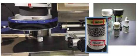
The lens and camera setup engineered by Xyntek with Opto Engineering lenses to image labels on vials
