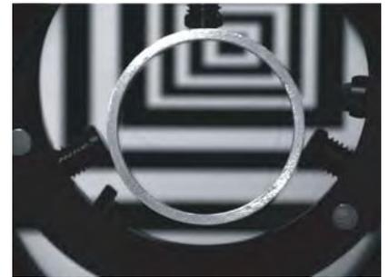
This effect is due to the specific path of the rays: in the case of common optics, any geometric information that is “parallel” to the main optical axis also shows a component on the detector plane direction, while in a telecentric lens this perpendicular component is totally absent.
