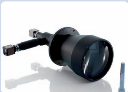
A TCDP4X144 imaging a screw with two different cameras
