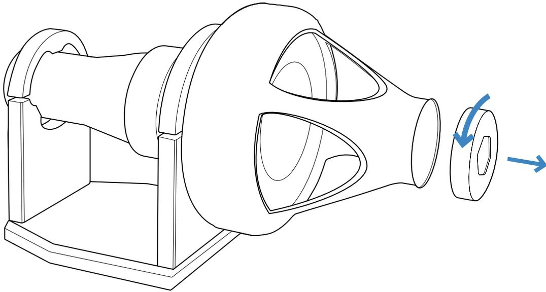
1 Remove PCMPMIRR mirror array by unscrewing it
