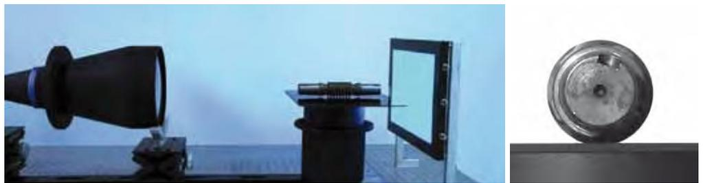
Opto Engineering® lenses bi-telecentricity also yields even illumination of the detector, which proves useful in several applications such as LCD, textile, and printing quality control. Moreover, when integrating dichroic filters, bi-telecentricity assures that the ray fan axis strikes the filter normal to its surface thus preserving the optical band-pass throughout the entire image plane.
