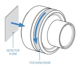
Rotate the focusing knob **clockwise** to move the lenses **away** from the detector, and focus objects **closer to the optics**.
