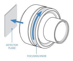
Rotate the focusing knob **counter-clockwise** to move the lenses **closer to the detector**, towards **infinity** position.
