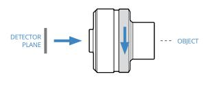
Once you have achieved the best focus position, lock the barrel in place by simply screwing the locking pin with an M1.5 Allen key.
